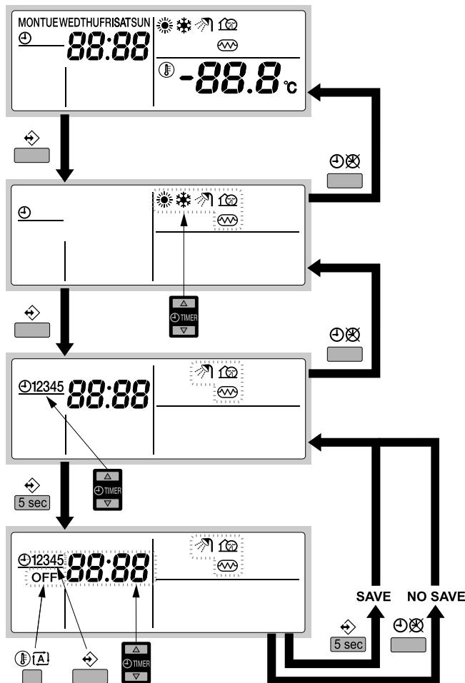
Programming domestic water heating, booster heater or quiet mode is carried out as follows:
